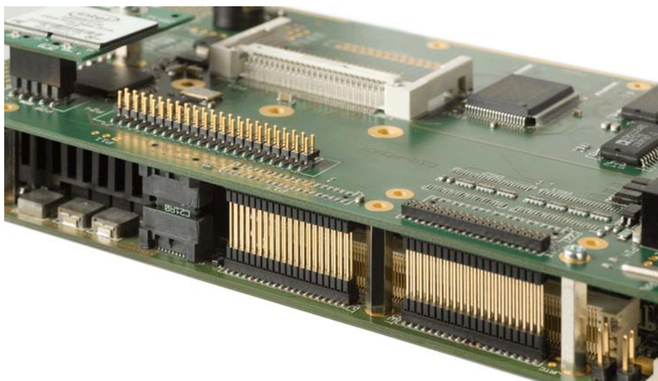
Mezzanine Expansion Connectors
