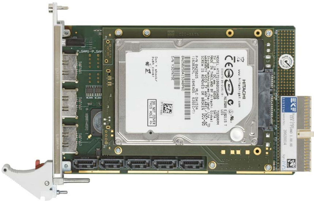
CE4-PIANO with C20-SATA Dual Drive Mezzanine Top View
