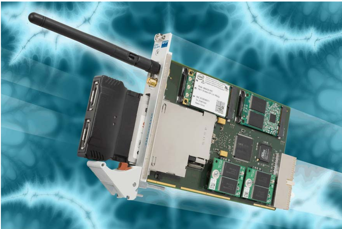
CP5-GLAM Populated with PCIe Mini Cards & USB SSDs
