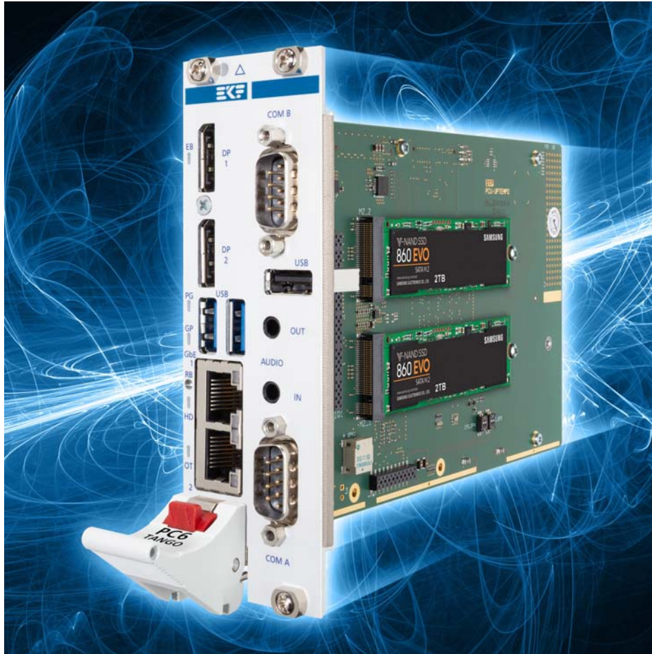
PC6-TANGO w. PCU-UPTempo (8HP F/P Assembly)
