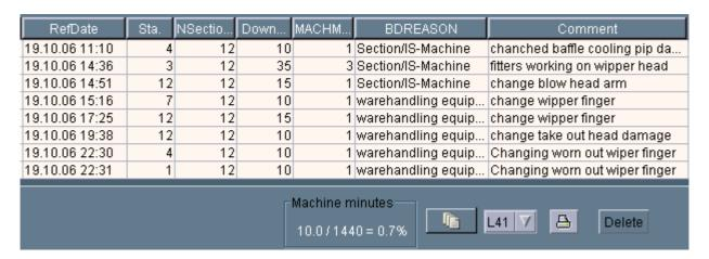
In case each section of IS machine delivers one pulse per "Gobs delivered", iAfis will record section efficiency automatically and also section stops automatically (in case section pulse pauses for >= 1 minute). See pictures how this data / events are shown:
