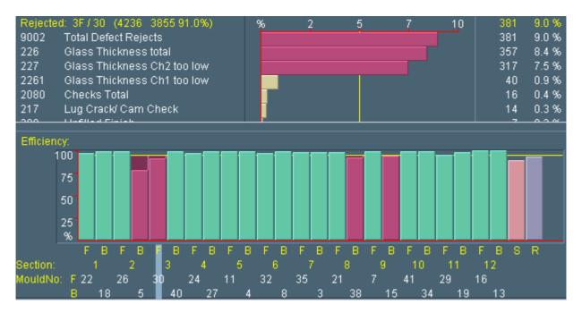
Also here with one mouse click the histogram for one defect and one section or mould can be displayed. As you can see, defect thickness decreased after replacement of Blow mould, Baffle arm, Plunger and Thimble.
