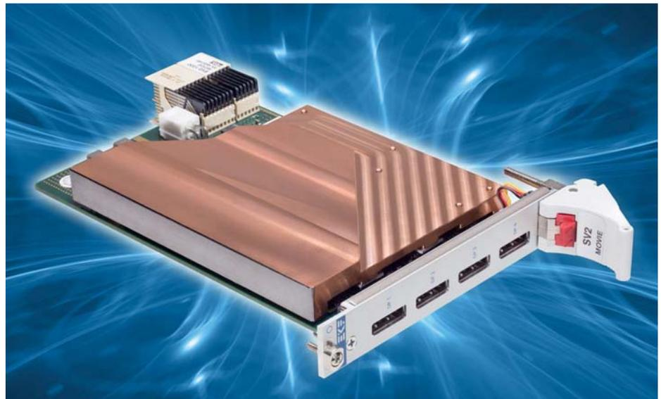
**Pic.4:** The entire waste heat of this video module is collected and transferred to the upper end surface (bottom left in the picture)
