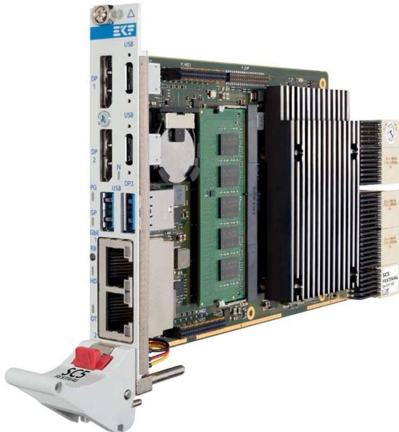
**Pic.1:** A complete XEON 3 industrial computer with all the usual peripherals on a single euroboard of 3U and with only one slot space requirement (4HP).
